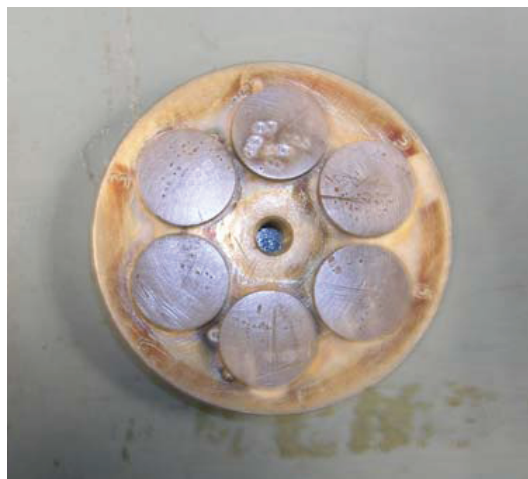
Figure 3.5: Target carousel loaded with six steel targets with varying carbon concentrations.
