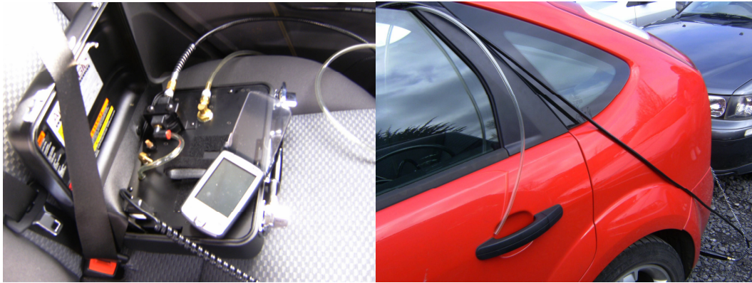
Figure 3.27: gas analyzer fitted in the car
