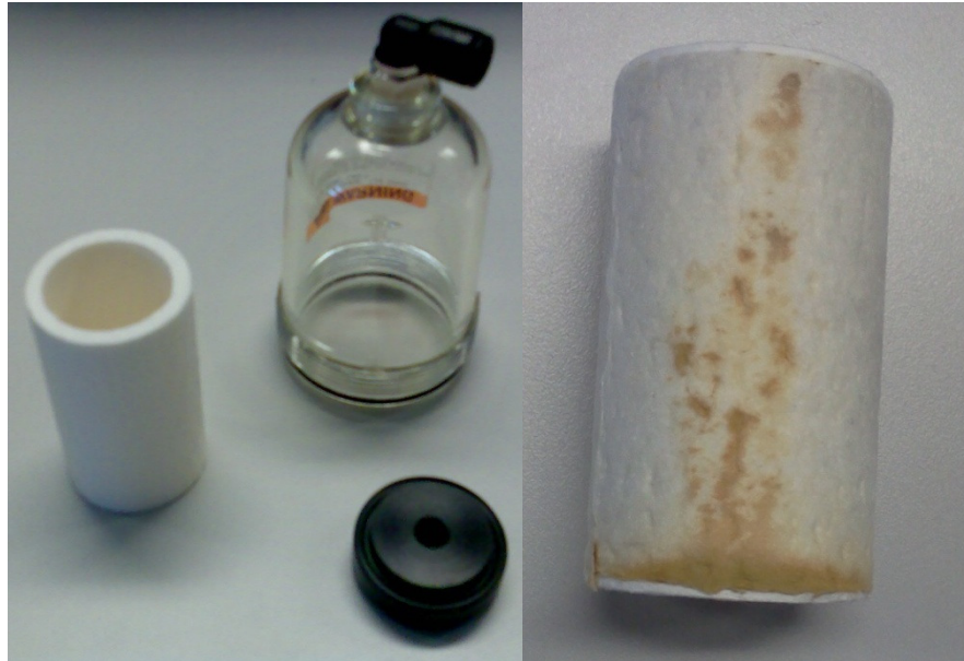
Figure 4.28: The water trap filter has been used and replaced (left image) with a newer version with the housing (right image).
