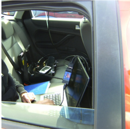
Figure 4.27: OBD scan tool connected to both car and laptop.
