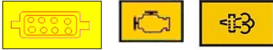
Figure 2.14: Blocked DPF warning lights [22]
