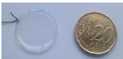
Figure 3.10: Novel Passive sampling disk. Passive sampling membranes cast from glass cylinder pre exposure (left) (21 mm * 0.2 mm); 20 cent coin for size comparison (right)
