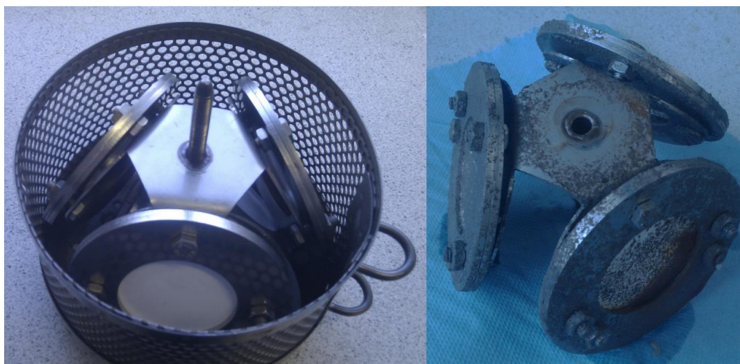
Figure 5.2: POCIS samplers before (left) and after (right) 32 day exposure in Ringsend (October-November 2011)
