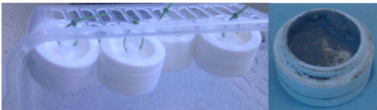
Figure 5.1: Non-polar Chemcatcher samplers before (left) and after (right) 32 day exposure in Ringsend (October-November 2011)
