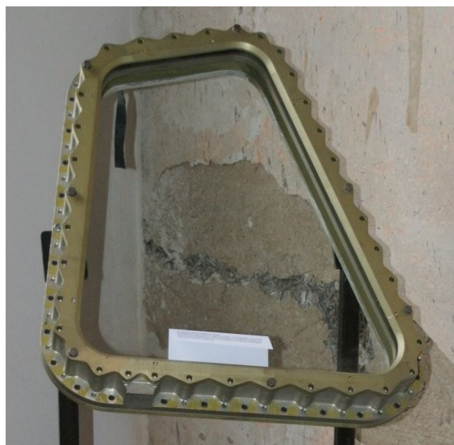
Photograph 7: Airtight pressurized window assembly from the cabin of Buran orbiter. Photograph credit: Weltraumladen.de.
