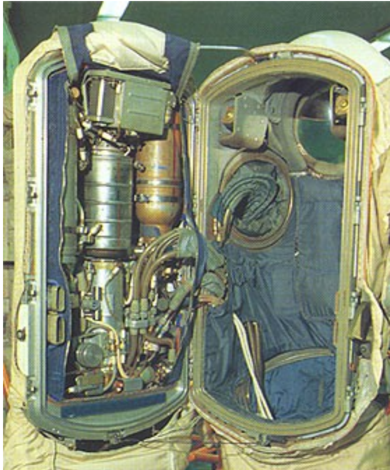
Photograph 6: Orlan's airtight hatch door and hatch frame from the website of NPP Zvezda. Photograph credit: OAO NPP Zvezda.
