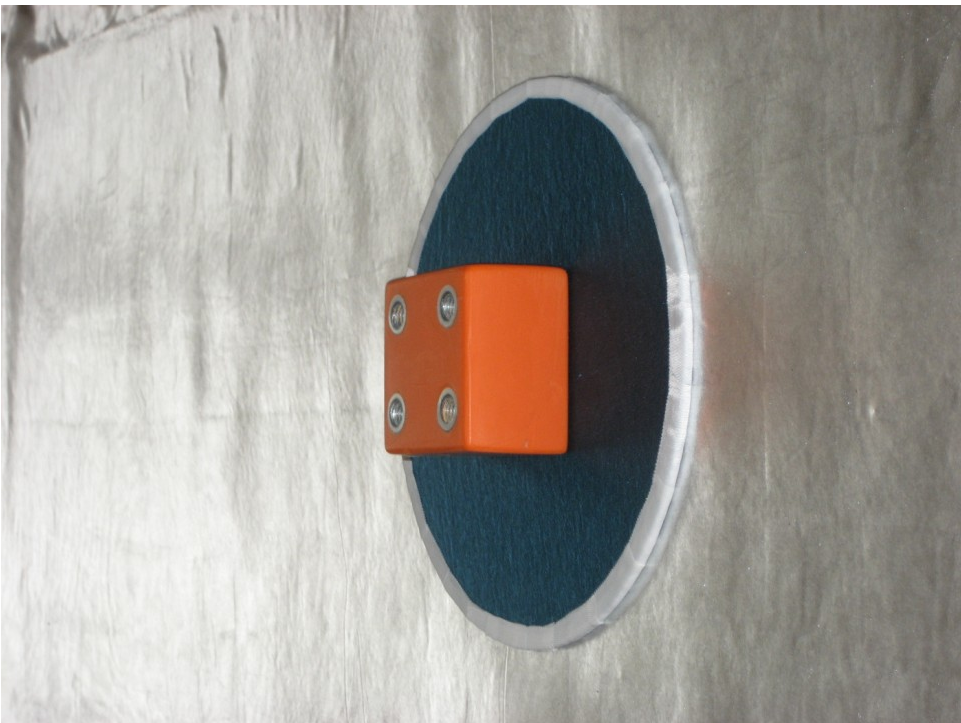
Photograph 5: Perspective view of the model of a structural load bridge component that has been installed into a soft airtight sack, showing the bridge component's one visible half, the other half is behind the soft airtight sack.
