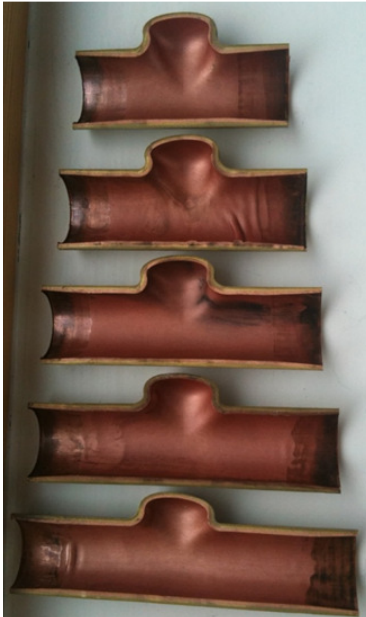
Figure 3.28: Bi-layered T-shape hydroformed parts from different tubes lengths.
