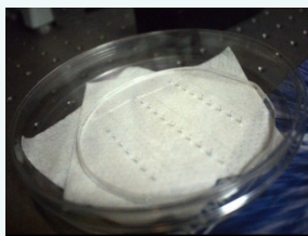
Fig.3 Many trenches can be arrayed on a single disc.
