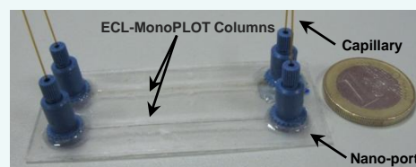
Figure 7. Resulting micro-fluidic chip with commercial nano-ports for connection of chip to external pumps via fused silica capillaries.
