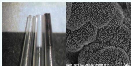
**Fig. 2:** (left): Image of PP tips incorporating AuNP-aggglomerated monolith at various stages of preparation. (right): Fe-SEM image of AuNP-aggglomerated polymer monolith (60,000x)
