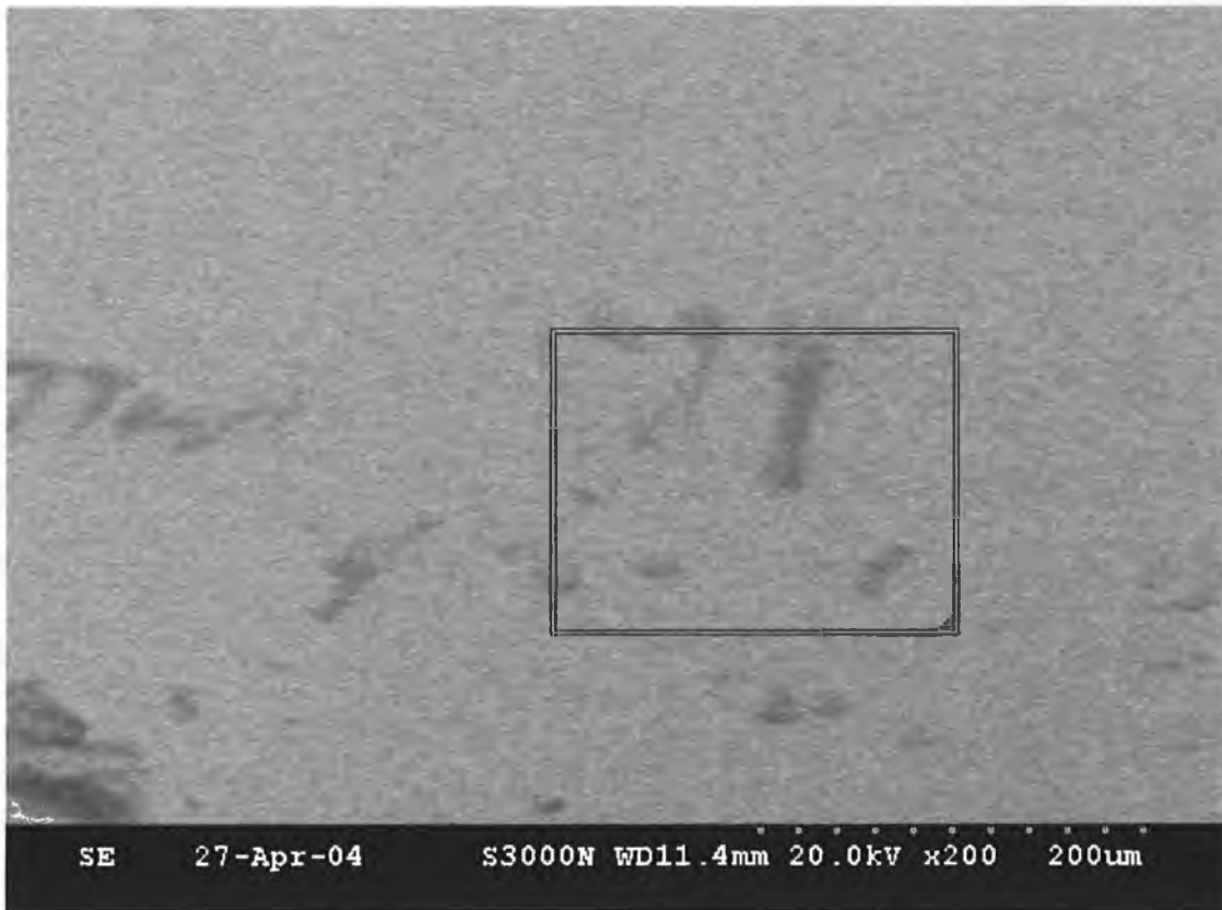
Figure 5.9 SEM image of a 1.25mm radius copper macroelectrode. The image was taken at a working distance of 11.4mm, beam energy of 20kV and a magnification of 200.
