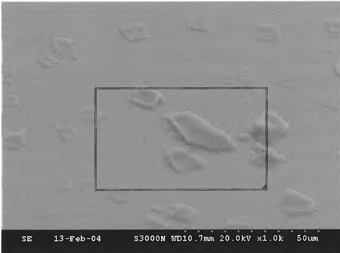
Figure 5.10 SEM image of a 1.25mm radius copper macroelectrode. The image was taken at a working distance of 10.7mm, beam energy of 20kV and a magnification of 1000.
