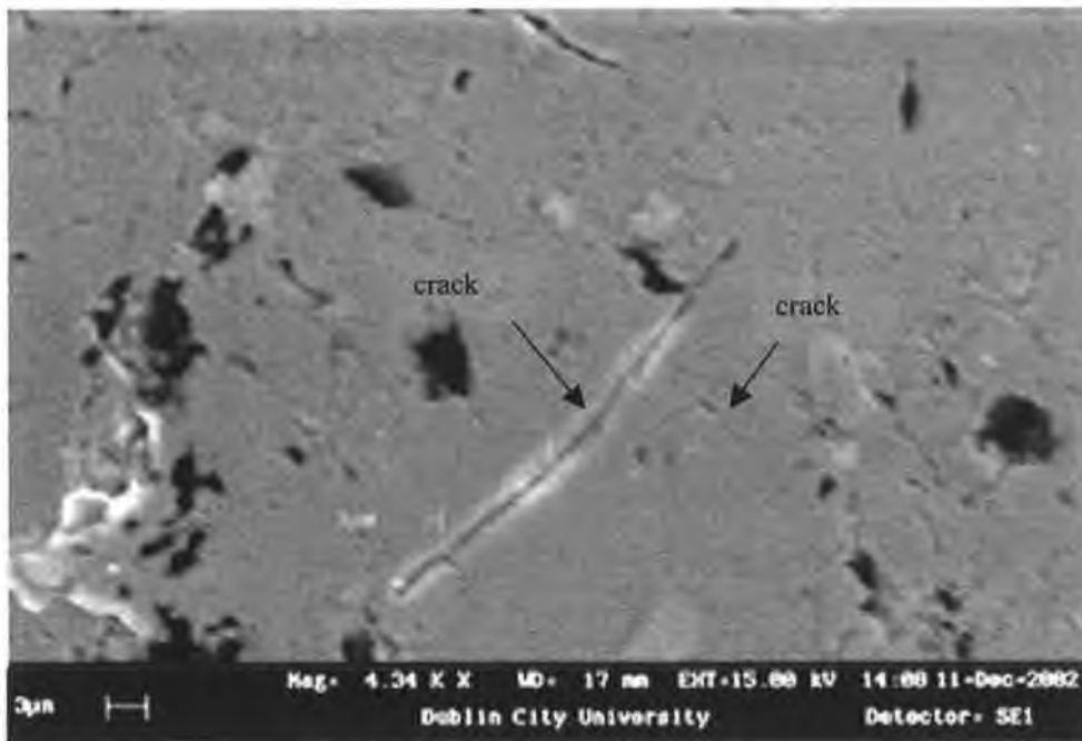
Figure 7.4: Typical SEM micrograph shows cracks obtained during the four point bend test of DLC film ( 1.5 \times 10^{-3} mbar, 1 A and 100% C_2H_2 gas).
