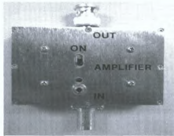
Figure 4.5: 20dB shielded amplifier designed for EMC measurements.
