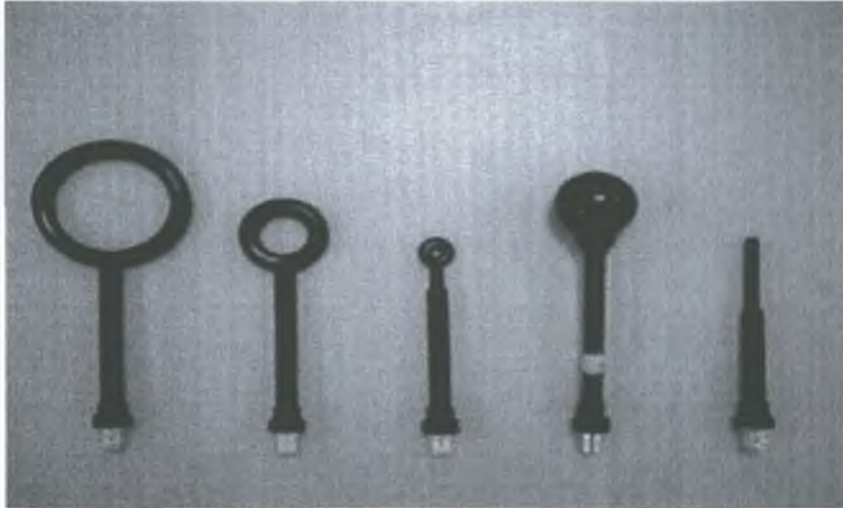
Figure 4.4: Five antennas lined side by side for comparison. The three loops pick up magnetic fields while blocking electric fields, while the ball and the monopole pick up electric fields while blocking magnetic fields. The different sizes allow for more (smaller) or less (larger) precise localisation of the offending emission.
