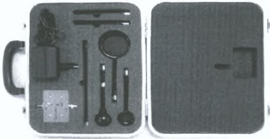
Figure 4.3: The EMC kit used to capture and amplify the radiated emissions emanating from the DUT.
