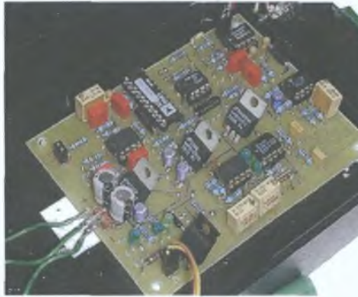
Figure 4.9: A photograph of the electronic circuit used in the LED-based prototype sensor system.
