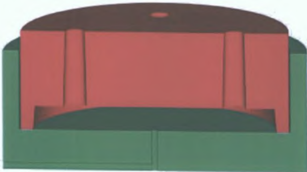
Figure 3-1: Section of the assembled PTFE mould.
