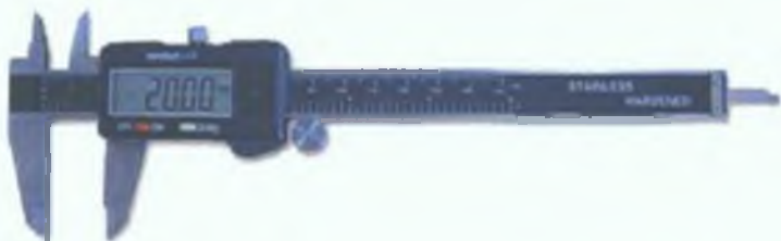
Figure 3-20: Vernier calipers used to measure the penetration of bone cement.
