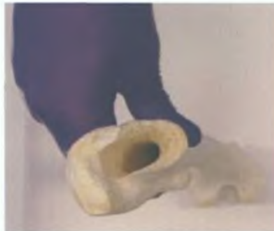
Figure 3-15: Prepared femur bone to start bone cement injection.
