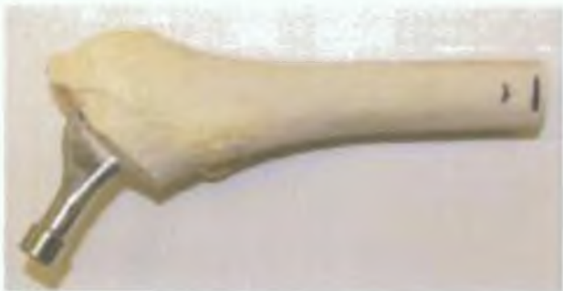
Figure 3-18: Femur bone cut at a distance of 17 cm below the femur head.
