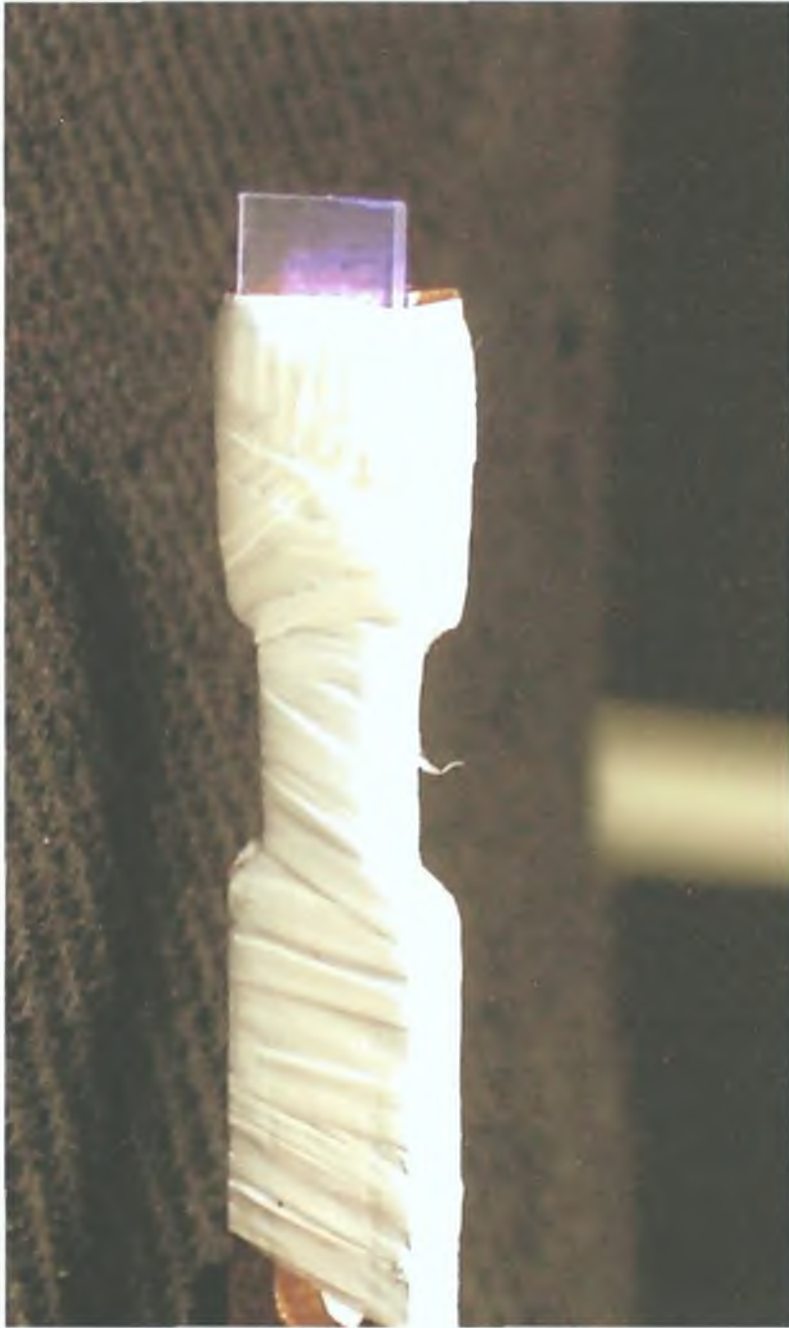
Figure F.3: Image of the PLD sample with a stripe excitation area in room light. Also shown is the sample holder.
