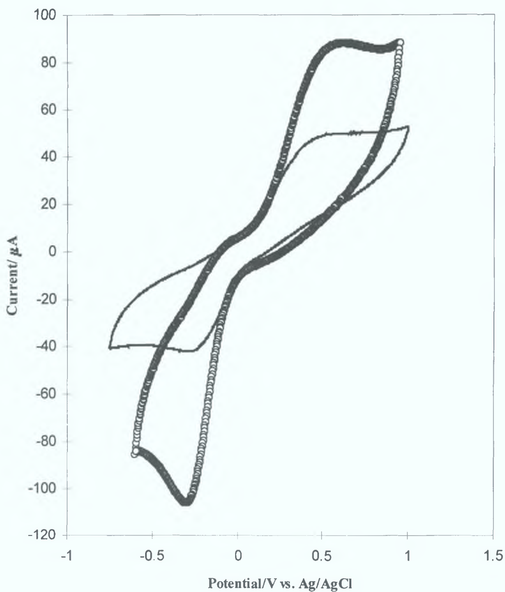
Figure 5.3. Cyclic voltammogram of (□)streptavidin-carbon-polymer and (—) avidin-carbon-composite in 1.81 mM hydroquinone with 0.1M KCl in 0.1 M phosphate buffer, pH 7.4. A Ag/AgCl reference electrode and a platinum auxiliary electrode were used. Initial potential was -0.6 V in a positive direction.
