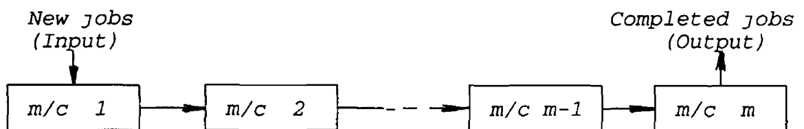
Figure 3.3: Job work-flow through machines in a pure flow-shop environment.
