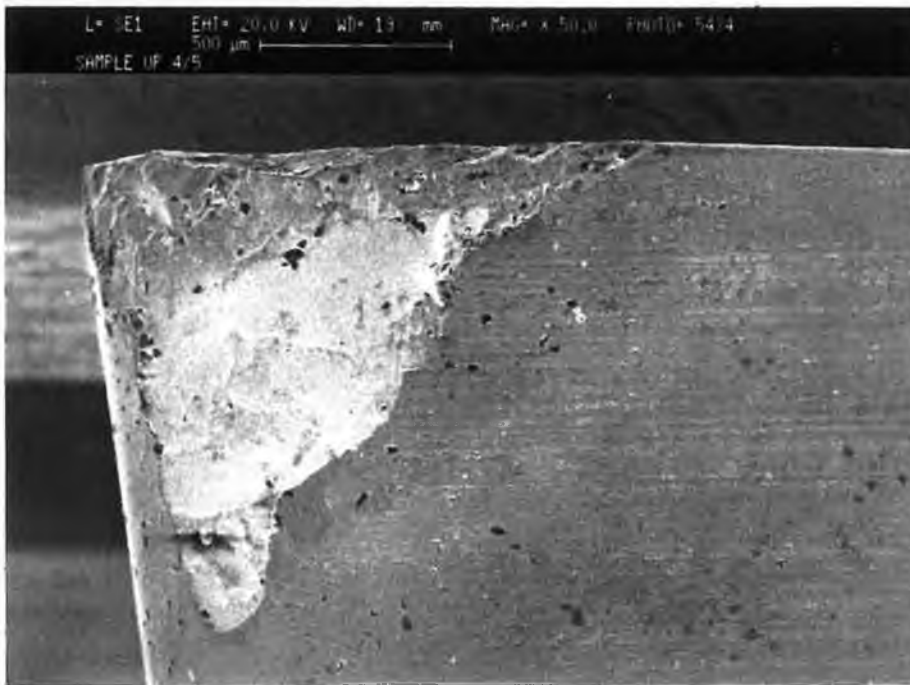
Fig.3: SEM image of the flank wear (VB2/VB3) of the carbide insert ( after 10 minutes) in full immersion end milling Inconel 718 at v = 19.32 m/min, f_z = 0.091 mm/tooth and a_a = 1.00 mm
