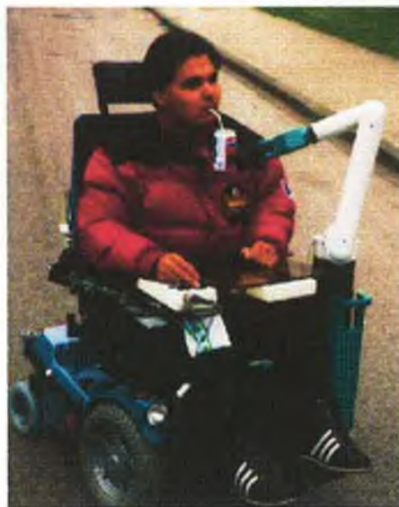
Figure 3.6-2 A Disabled Man using a Manus Robotic Arm
