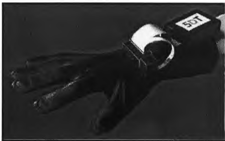
Figure 2.5: A typical VR Data Glove.
