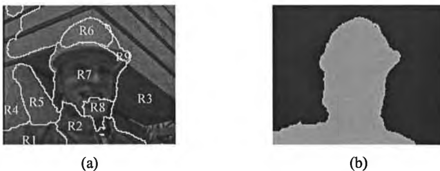
Figure 6-1: (a) Motion segmentation for the image. (b) Object segmentation by region merging, the semantic object shape is given by R1+R2+R8+R7+R6+R9 .
