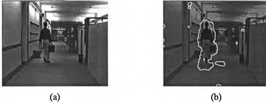
Figure 5-10: Results of the EM-MDL framework for motion segmentation (Hall Monitor). The only moving object is the man walking down the corridor. Affine motion models were used.
