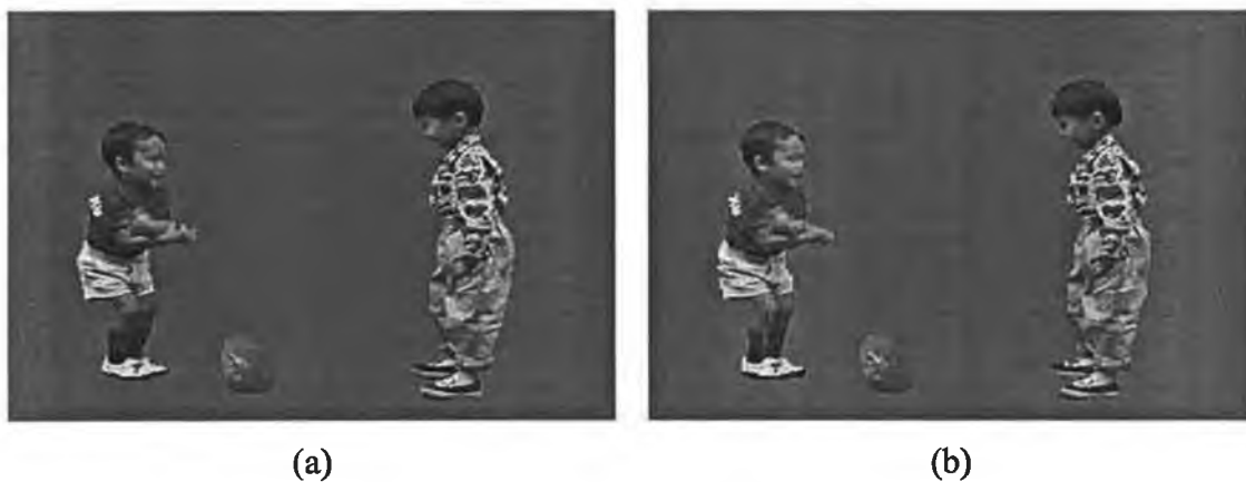
Figure 3-11: Illustration of shape distortions. (a) coded VOP with lossless shape, (b) coded VOP with lossy shape.
