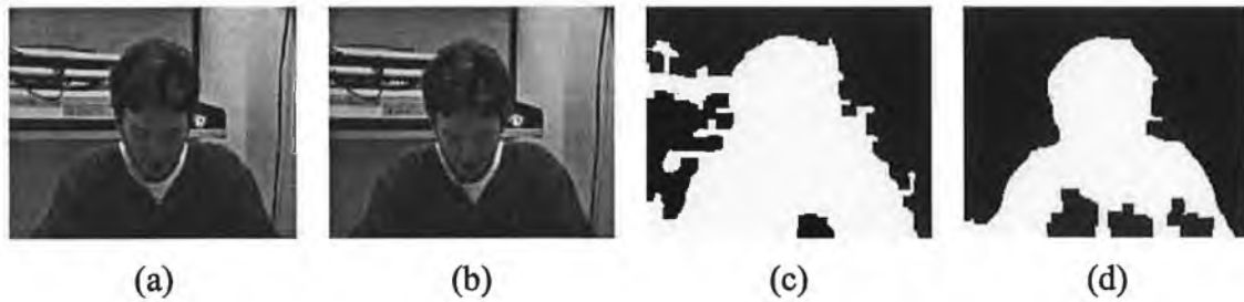
Figure 2-5: (a) and (b) are consecutive frames of a 8.33Hz sequence exhibiting illuminatory/noise variations. (c) shows the result of the change detection process with a threshold of 2, while (d) is the change detection mask with a threshold of 3.
