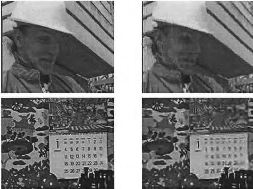
Figure 2-1: Artefacts in low bit-rate block-based video. On the left are high quality video frames and on the right are the same frames coded at very low bit-rate. Distortion takes the form of blur, blockiness (see top-right) and “mosquito” effects (see the noise close to contours of the ball and the train in the bottom-right image).
