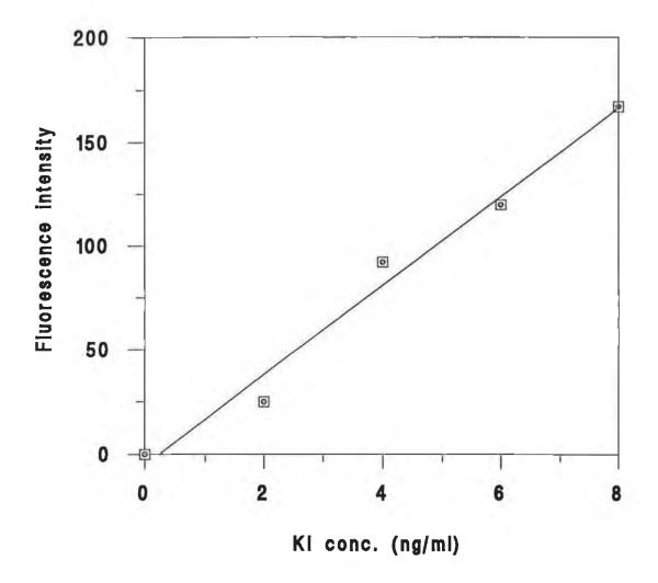
Figure 3.17 Graph of fluorescence intensity plotted against concentration of potassium iodide standards assayed in the optimised cerium(III) fluorimetric microassay.
