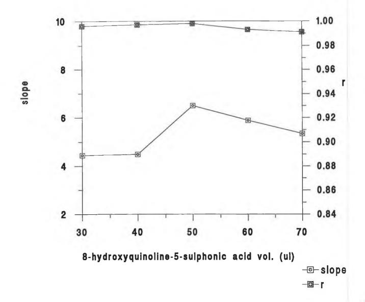
Figure 3.21 Effect of 8-hydroxyquinoline-5-sulphonic acid volume on the slope and correlation coefficient (r) of the graph of fluorescence intensity plotted against concentration for potassium iodide standards assayed in the cerium(IV) - 8-hydroxyquinoline-5-sulphonic acid fluorimetric microassay.
