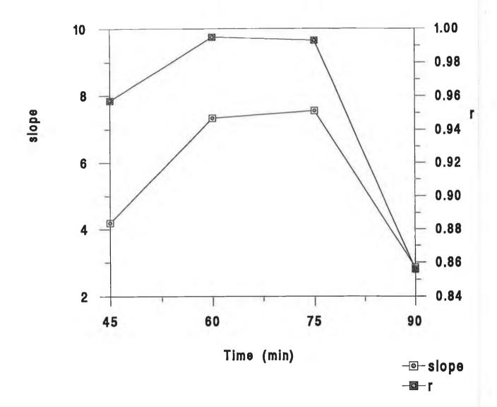
Figure 3.19 Effect of incubation period on the slope and correlation coefficient (r) of the graph of fluorescence intensity plotted against concentration for potassium iodide standards assayed in the cerium(IV) - 8-hydroxyquinoline-5-sulphonic acid fluorimetric microassay.
