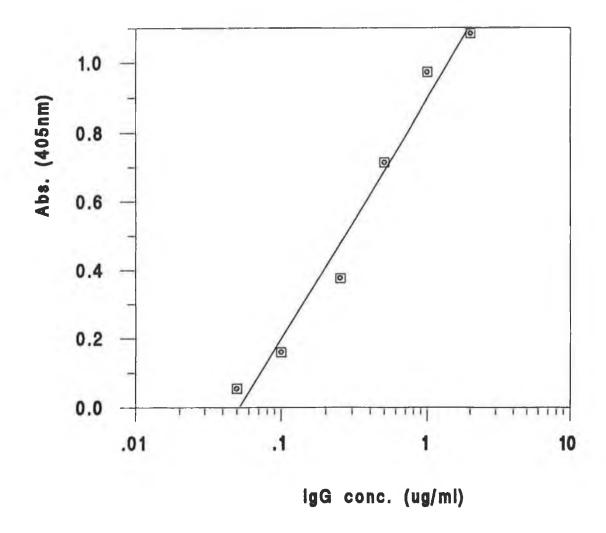
Figure 5.8 Graph of absorbance at 405nm plotted against concentration of human IgG standards assayed in an immunoassay using biotinylated HRP.
