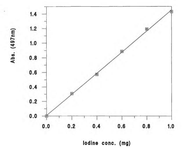
Figure 3.10 Graph of absorbance at 497nm plotted against iodine concentration, following treatment of potassium iodide standards with cerium(IV) and extraction of the liberated iodine into toluene.
