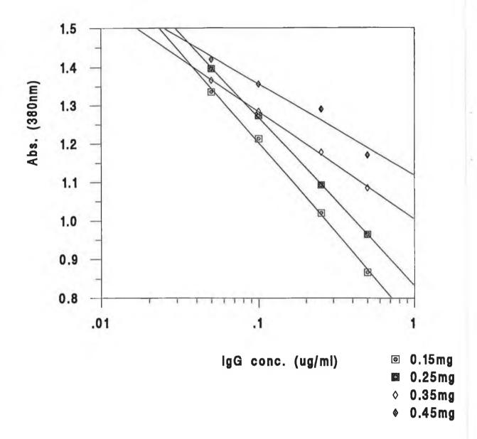
Figure 5.3 Graph of absorbance at 380nm plotted against concentration of human IgG standards assayed in an immunoassay using avidin labelled with various amounts of IBHR.
