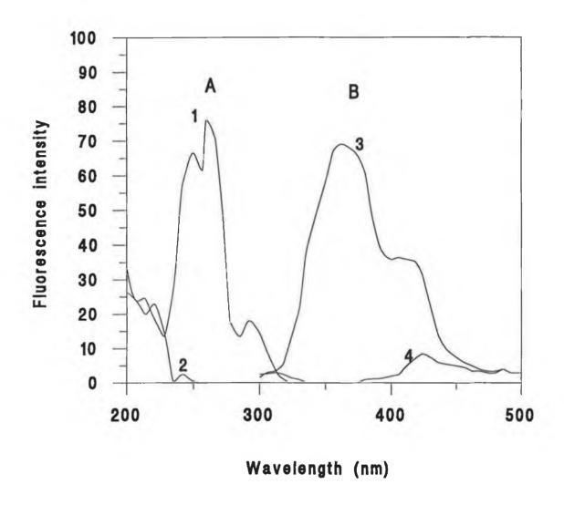
Figure 3.12 Fluorescence spectra for cerium(III): A, excitation and B, emission.
