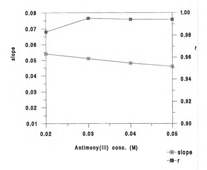
Figure 3.4 Effect of antimony(III) concentration on the slope and correlation coefficient (r) of the graph of absorbance plotted against concentration for potassium iodide standards assayed in the cerium(IV) - antimony(III) spectrophotometric microassay.
