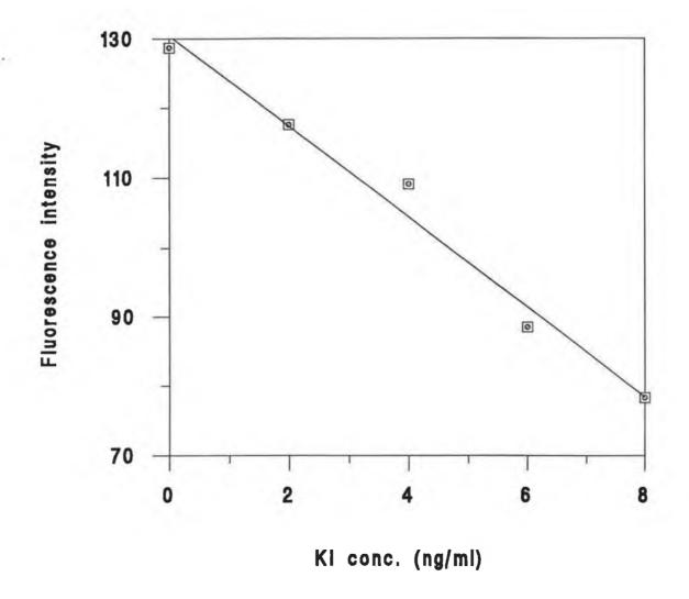
Figure 3.22 Graph of fluorescence intensity plotted against concentration of potassium iodide standards assayed in the optimised cerium(IV) - 8-hydroxy-quinoline-5-sulphonic acid fluorimetric microassay.
