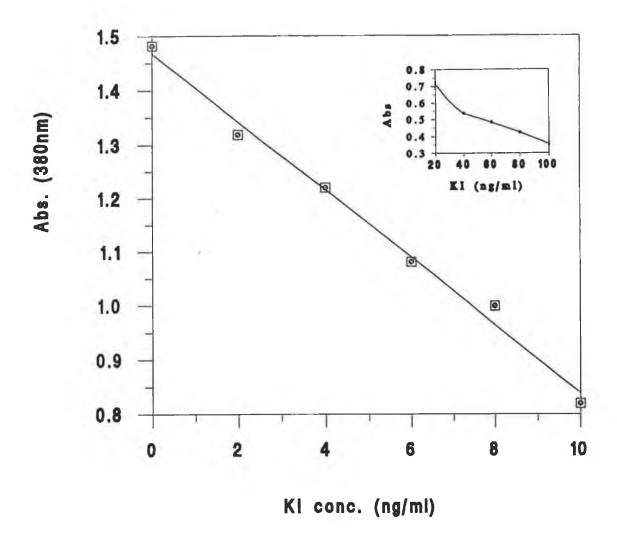
Figure 3.6 Graph of absorbance at 380nm plotted against concentration of potassium iodide standards (0 to 10ng/ml) assayed in the optimised cerium(IV) - antimony(III) spectrophotometric microassay.
