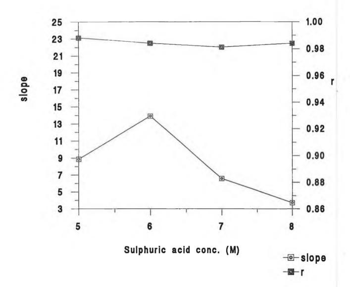
Figure 3.15 Effect of sulphuric acid concentration on the slope and correlation coefficient (r) of the graph of fluorescence intensity plotted against concentration for potassium iodide standards assayed in the cerium(III) fluorimetric microassay.
