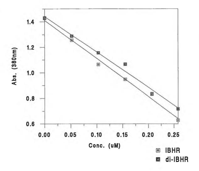
Figure 3.11 Graph of absorbance at 380nm plotted against concentration for IBHR and di-IBHR standards assayed in the cerium(IV) - antimony(III) spectrophotometric microassay.
