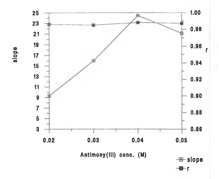
Figure 3.16 Effect of antimony(III) concentration on the slope and correlation coefficient (r) of the graph of fluorescence intensity plotted against concentration for potassium iodide standards assayed in the cerium(III) fluorimetric microassay.
