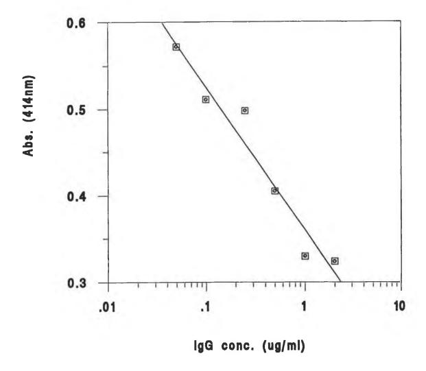
Figure 4.5 Graph of absorbance at 414nm plotted against concentration of human IgG standards assayed in a two-site immunoassay, using IBHR-labelled antibodies detected by the Sandell-Kolthoff reaction.
