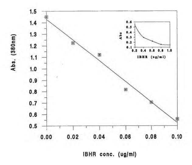
Figure 3.7 Graph of absorbance at 380nm plotted against concentration of IBHR standards assayed in the optimised cerium(IV) - antimony(III) spectrophotometric microassay. The insert displays the graph of absorbance at 380nm plotted against concentration of IBHR standards in the range 0.2 to 1ug/ml.
