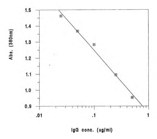
Figure 5.4 Graph of absorbance at 380nm plotted against concentration of human IgG standards assayed in an immunoassay using IBHR-labelled avidin.
