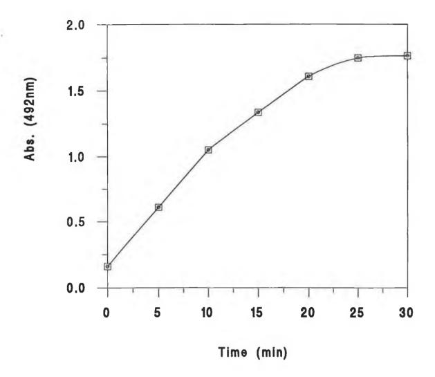
Figure 4.2 Graph of absorbance at 492nm plotted against time, for measurement of the enzyme activity of HRP-labelled antibodies.
