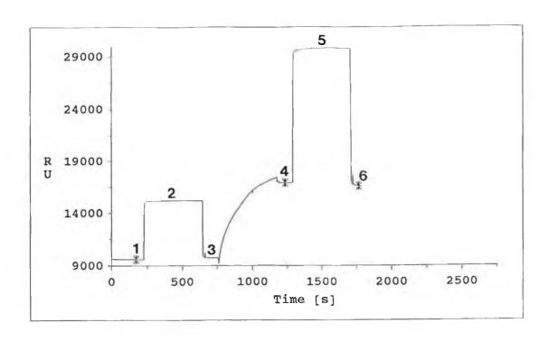
Figure 4.7 An example of a sensorgram showing the immobilisation of human IgG onto the activated surface of a sensor chip.
