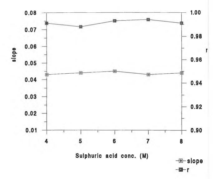
Figure 3.3 Effect of sulphuric acid concentration on the slope and correlation coefficient (r) of the graph of absorbance plotted against concentration for potassium iodide standards assayed in the cerium(IV) - antimony(III) spectrophotometric microassay.
