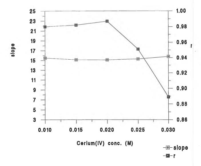
Figure 3.14 Effect of cerium(IV) concentration on the slope and correlation coefficient (r) of the graph of fluorescence intensity plotted against concentration for potassium iodide standards assayed in the cerium(III) fluorimetric microassay.
