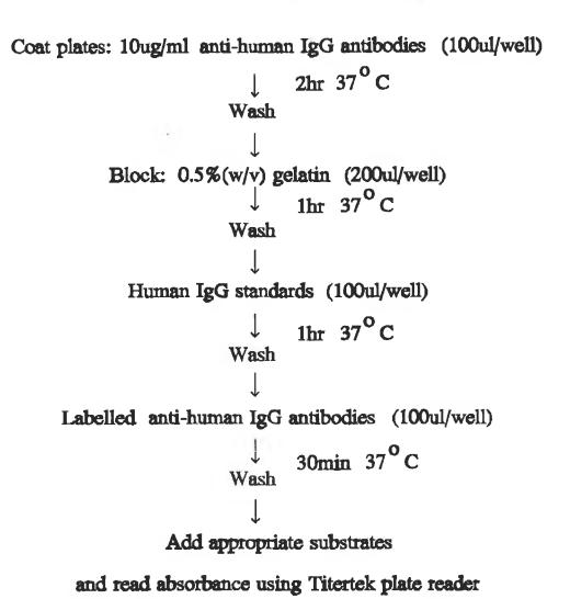
Figure 4.3 Flow diagram of the two-site immunoassay using IBHR- or HRP-labelled antibodies. (A detailed description of the protocol is given in Section 2.6.1)
