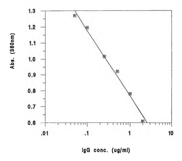
Figure 4.4 Graph of absorbance at 380nm plotted against concentration of human IgG standards assayed in a two-site immunoassay, using IBHR-labelled antibodies detected by the cerium(IV) - antimony(III) reaction.
