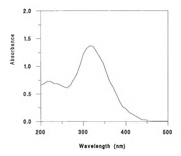
Figure 3.1 Absorbance spectrum of ceric ammonium sulphate in 6M H<sub>2</sub>SO<sub>4</sub>.
