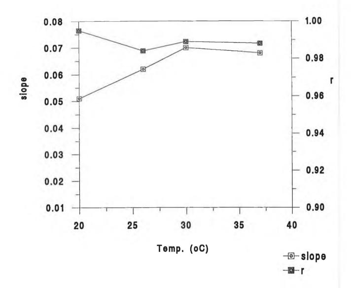
Figure 3.5 Effect of temperature on the slope and correlation coefficient (r) of the graph of absorbance plotted against concentration for potassium iodide standards assayed in the cerium(IV) - antimony(III) spectrophotometric microassay.
