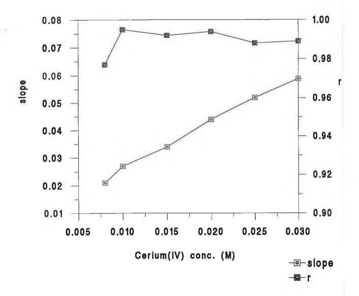
Figure 3.2 Effect of cerium(IV) concentration on the slope and correlation coefficient (r) of the graph of absorbance plotted against concentration for potassium iodide standards assayed in the cerium(IV) - antimony(III) spectrophotometric microassay.
