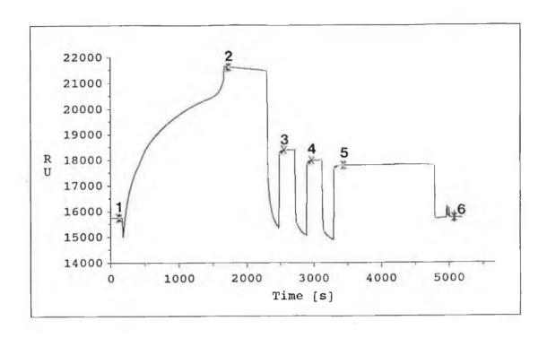
Figure 4.8 An example of a sensorgram showing the interaction between human IgG immobilised on the surface of a sensor chip, and native anti-human IgG antibodies.
