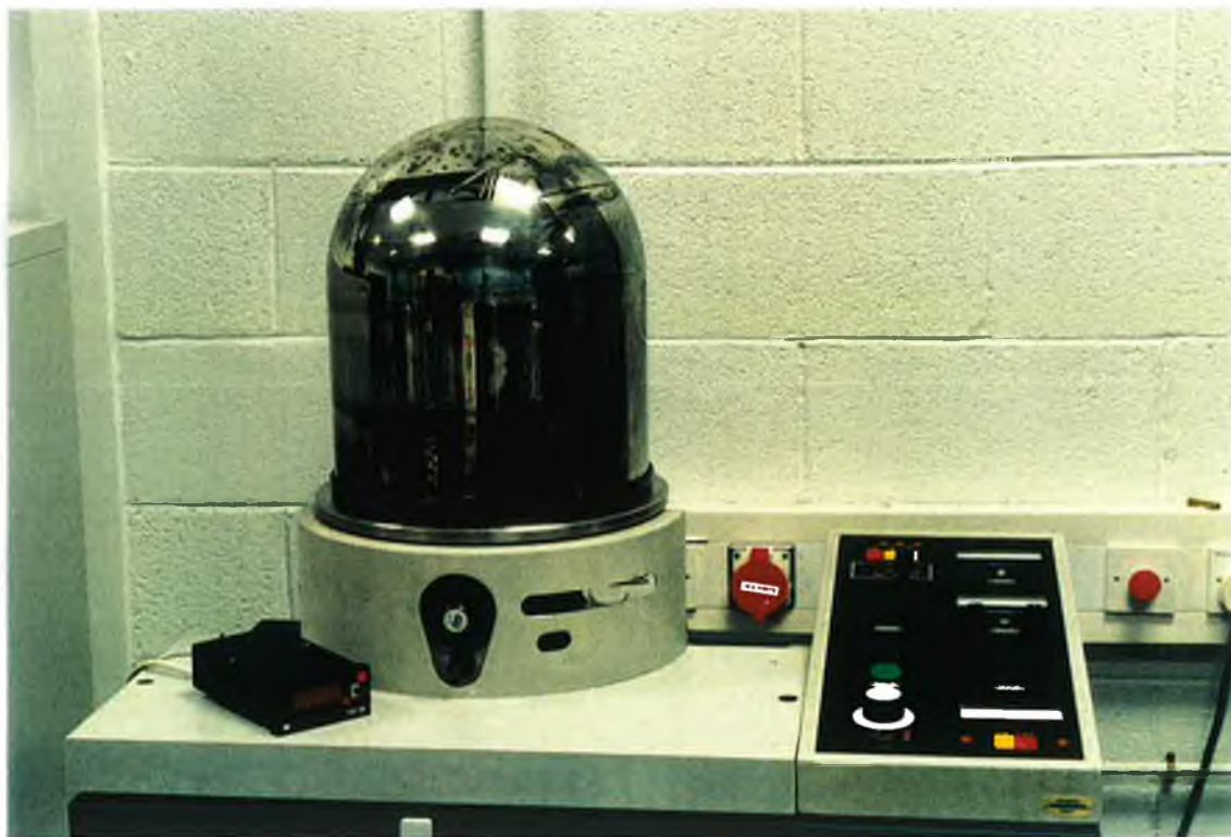
Figure 7: (c) The complete post-annealing system with cover (bell jar).
