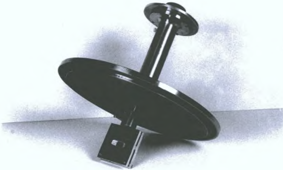
Photograph B.3 The multilayer and mount attached to a rotatable shaft with angular calibration.
