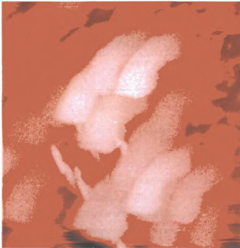
Figure 6.9 : STM image of an untreated Germanium sample.
