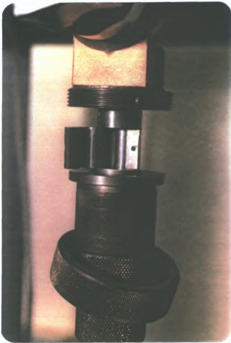
Plate 4.3 Shows the projectile position inside the loading throat.
