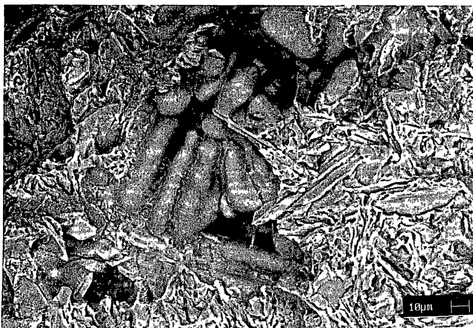
Figure 4 25 Tensile fracture surface topography showing porosity content (form SEM)
