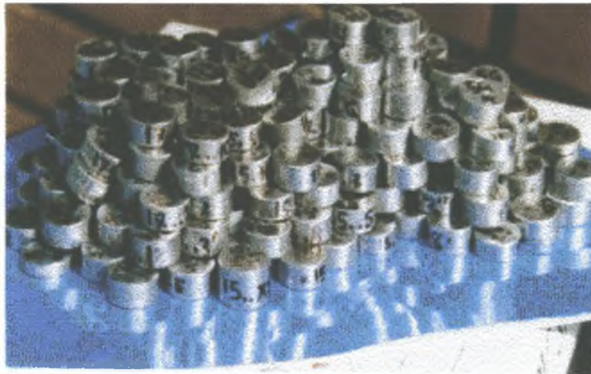
Figure 3.22 : Specimens from ingot type B, 18 mm diameter.
