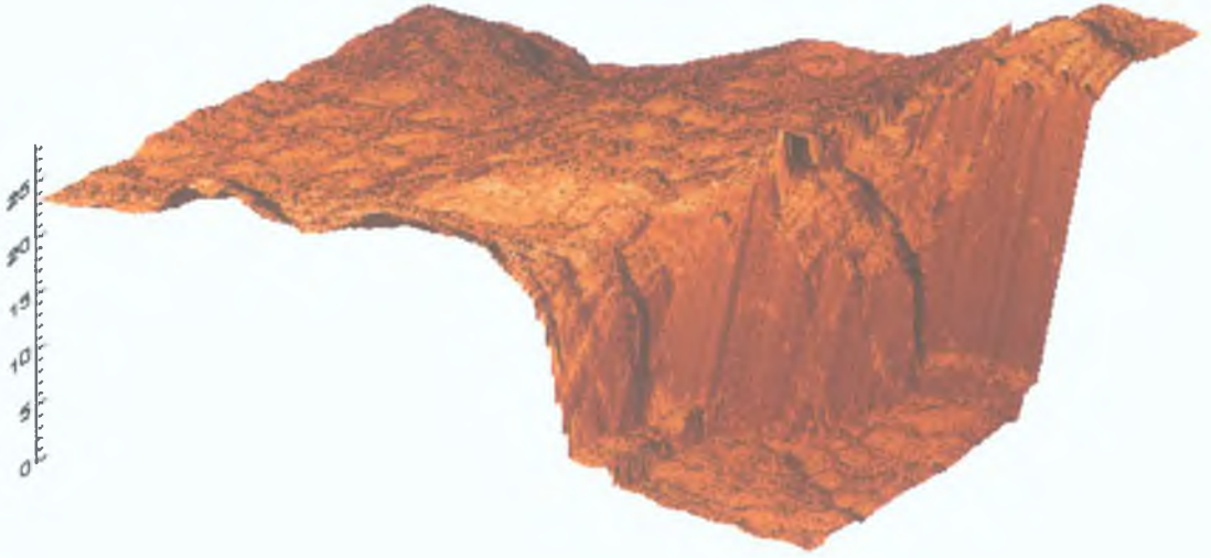
Fig 3.2. (160nm) 2 STM image of a cleavage step on an Au coated NaCl crystal, with the vertical range shown on the left in nm.
