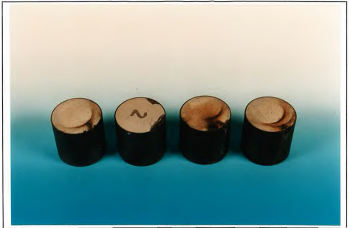
Plate 5.3 Photograph of varistor failure due to pin hole, puncture and flash-over during strength test.
