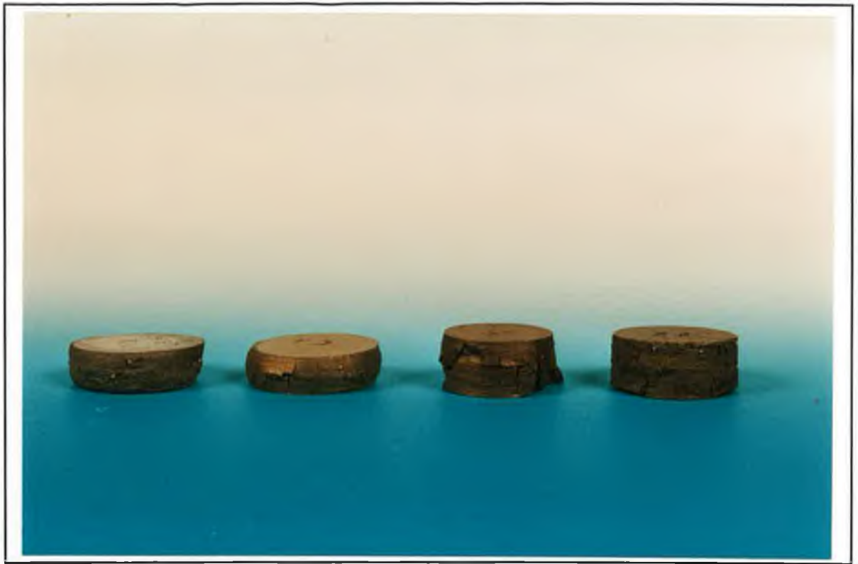
Plate 6.3 Photograph of fracture of Al-6061/SiC composites during compression test.
