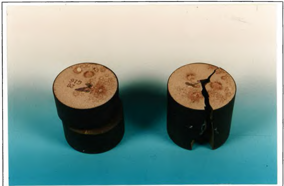
Plate 5.2 Photograph of varistor's failure in HASD test.
