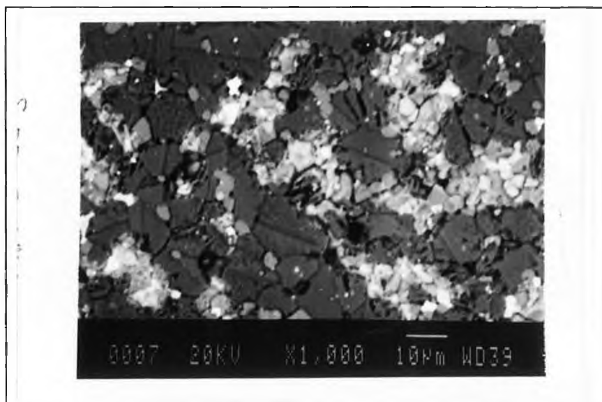
Plate 5.5 SEM photograph of the disc sintered by weight loss rate and shrinkage rate limit 3 g/kg/h and 10 \mu\text{m}/\text{mm}/\text{h} respe.
