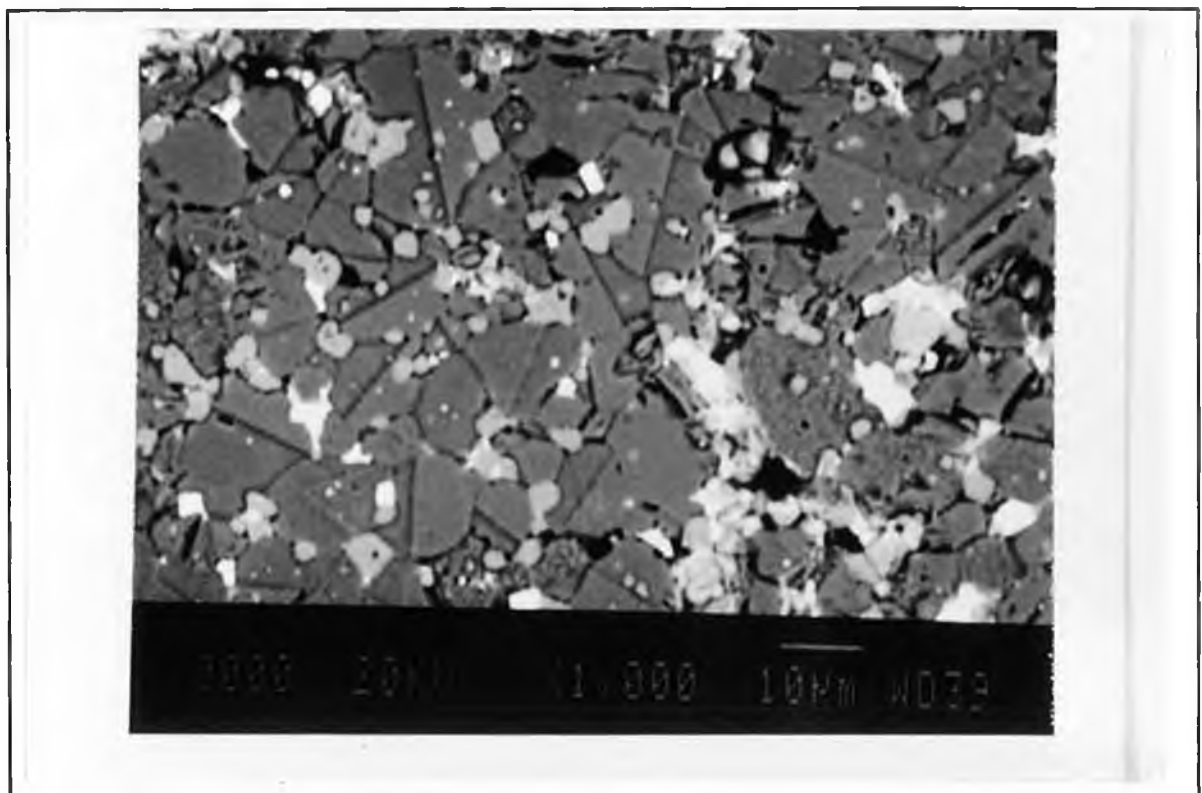
Plate 5.7 SEM photograph of the disc fired by weight loss rate and shrinkage rate limit 3 g/kg/h and 40 \mu\text{m}/\text{mm}/\text{h} .
