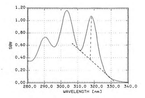
Fig. 2.1. UV absorption spectrum of Pimaricin showing measurement of peak height.
