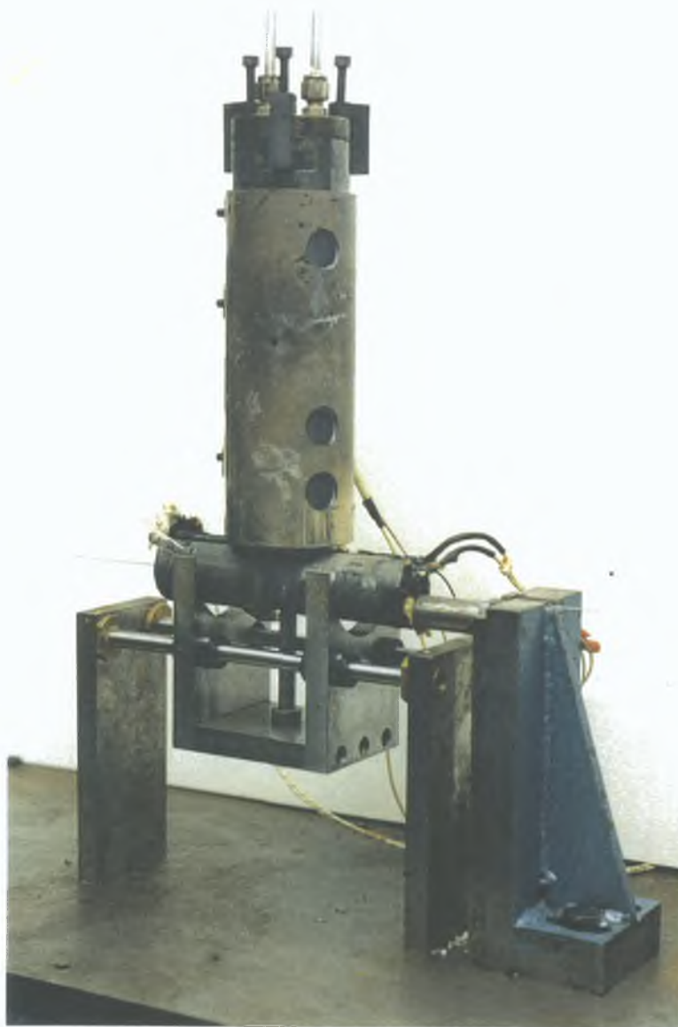
Plate 3.4. Melt chamber with leakage control and pressure unit(inside the heater band) and load cell
