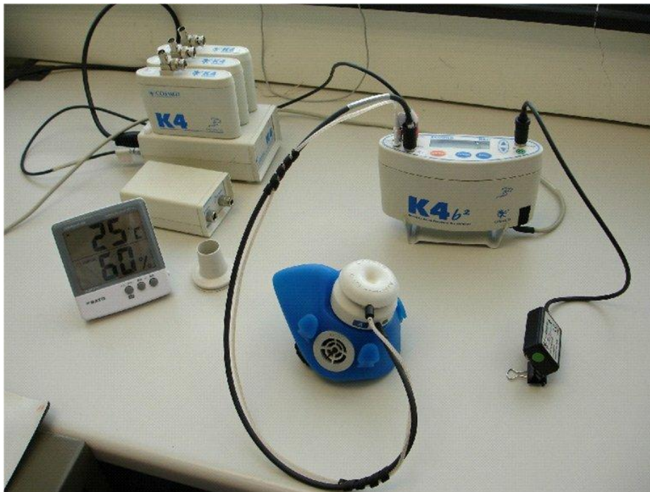
Figure 3.7: Cosmed k4b2 Metabolic Sensor
