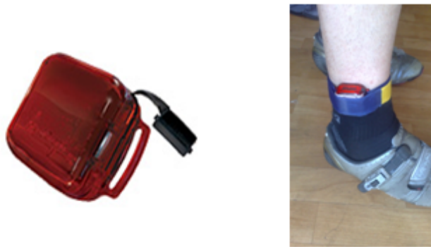
Figure 3.1: A GT3X accelerometer and its deployment on an ankle
