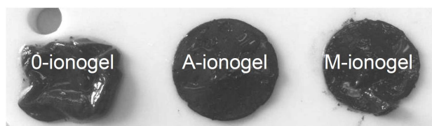
Figure 4-2. MIGs after removal from the moulds. Diameter is 15 mm.
