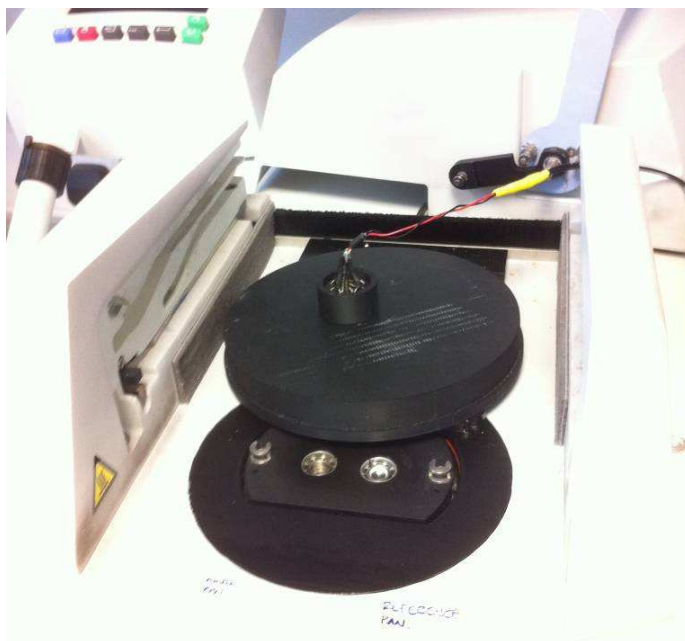
Figure A 1. The sample chamber and LED array holder printed with a 3D printer. Design by B.Z.
