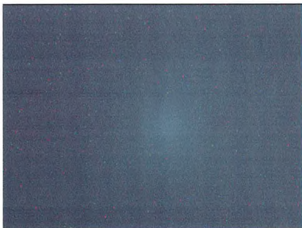
Figure 6.11: Picture of membrane 2 in buffer. Red, Green and Blue channel averages are 70.5, 65.2, and 84.0 respectively
