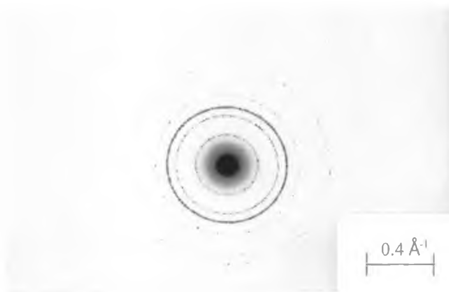
Figure 4.21: Selected area diffraction from a crystalline region.
