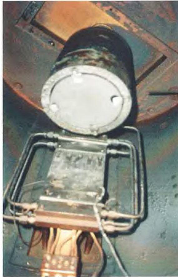
Figure 3.10: Heating plate inside the vacuum chamber. The top magnetron is also shown.
