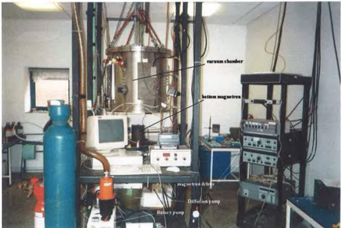
Figure 3.9: High vacuum system
