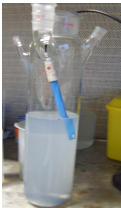
Figure 5-7 1L photoreactor after photodegradation using 1:1 IPCA, loose \text{TiO}_2 is visible in solution as a grey cloud. A pH probe is also present in the solution.
