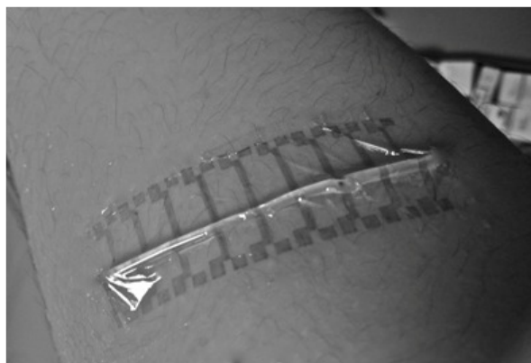
Figure 2.7. Concept of a flexible and conformal OEETs/ionogel array worn on the forearm. (adapted from reference [313])
