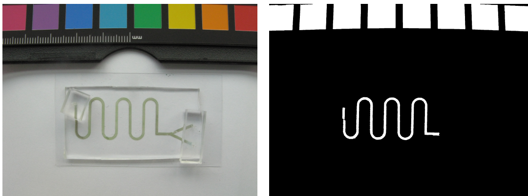
Figure B2. Picture of a captured image (left) during the experimental procedure showing the colour reference chart/patches and flow channel. Mask image (right) after image processing algorithms are applied.
