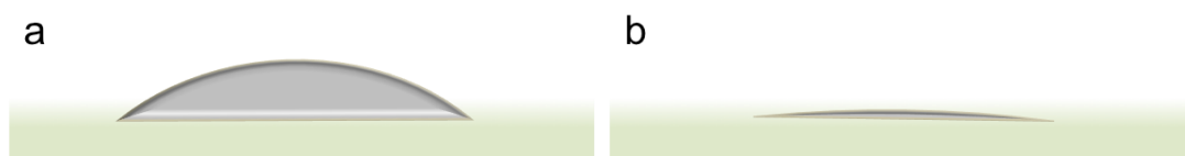
Figure 3.5. Schematic side view of a single actuator operated by a projector. (a) Large membrane deflection upon light illumination and pressure; (b) deflection erased by a second light illumination (no pressure applied). Adapted from [40].
