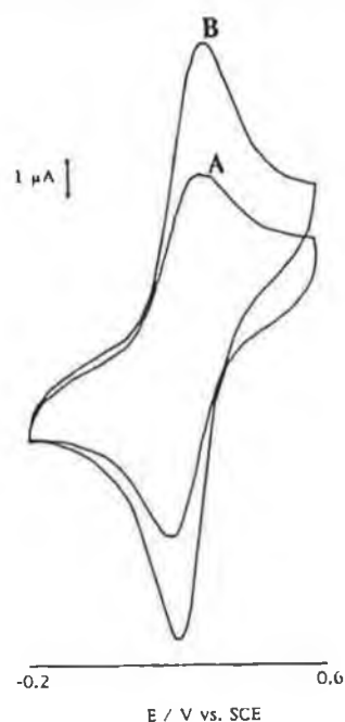
Fig. 2. Cyclic voltammograms of [\text{Os}(\text{bipy})_2(\text{PS})_{7.5}(\text{DMAP})_{2.5}\text{Cl}]\text{Cl} in A) 0.1 \text{ mol dm}^{-3} \text{ H}_2\text{SO}_4 and B) 10% v/v ethanol in 0.1 \text{ mol dm}^{-3} \text{ H}_2\text{SO}_4 , sweep rate: 0.10 \text{ V s}^{-1} .
