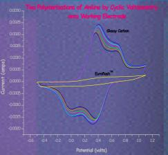
The two different carbon surfaces yield very different cyclic voltamograms after the same number of cycles. The very small amount of current passed for the Euroflash<sup>TM</sup> compared to the glassy carbon demonstrates a high charge transfer resistance for the manufactured strip.
