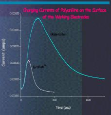
The graph shows the different charging currents of the polyaniline demonstrating the reduced deposition of the polymer on the Euroflash<sup>TM</sup> electrode.
