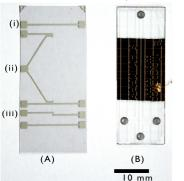
Figure 2: Layout of the screen printed upper piece (A) of the chip containing the reference (i) and auxiliary (ii) electrodes as well as the electrodes for C4D detection (iii).
