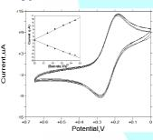
Figure 3: Cyclic voltamogramms (CVs) of ferrocyanide carried out inside the channel (100 mV/s)
