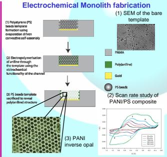
**Figure 4:** The fabrication of the reproducible microstructured poly(aniline) monolith is a 3 step process.
