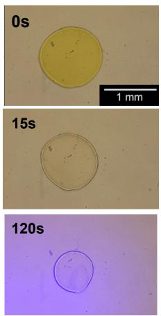
Drawback: These hydrogels function only in acidic conditions (HCl, pH~3)
