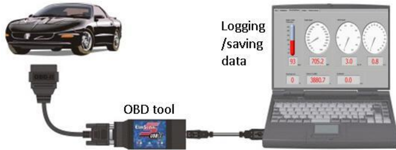
Fig.5. OBD scan tool connected to both car and laptop
