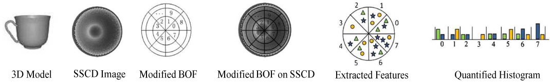
Figure 2.5, The illustration of the modified BOF method using SSCD proposed by Li et al. [31]
