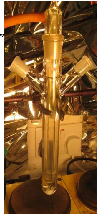
Figure 3-4: Photograph of photodegradation of dye/TiO 2 composite
