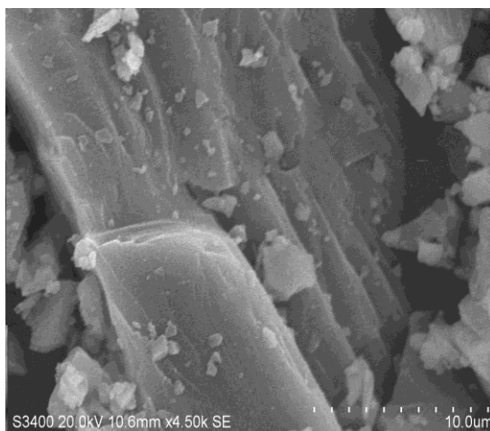
Figure 5-9: Bare dolomite imaged at 4.5k magnification
