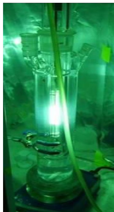
Figure 3-2: photograph of photodegradation of AC/TiO 2 composite
