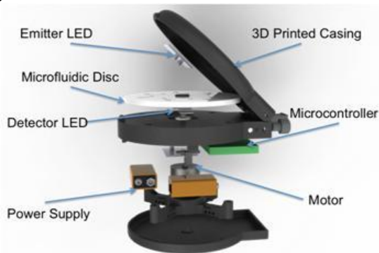
Fig. 2: Computer generated exploded view of the CMAS components.
