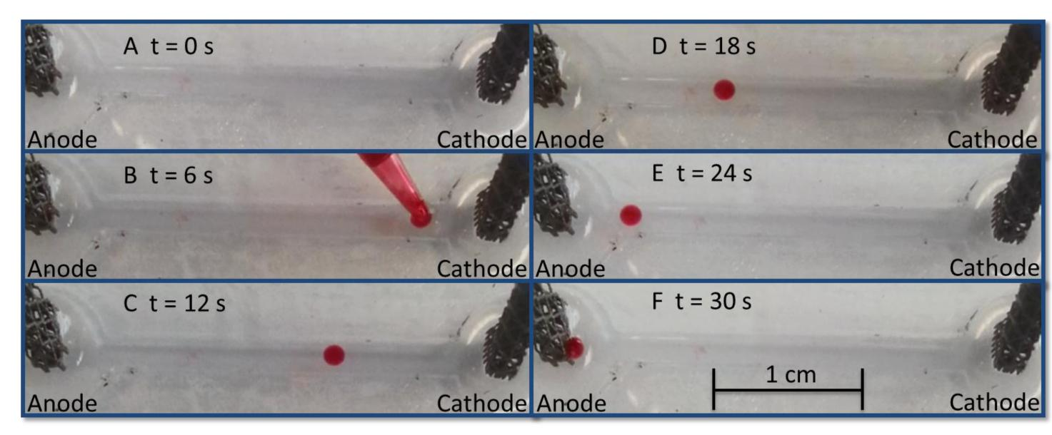
Once the voltage has been applied to the solution, the mobile cations migrate towards the cathode (Na<sup>+</sup> ions towards the starting position) and the mobile anions migrate toward the anode (Cl<sup>-</sup> ions towards the destination), creating a Cl<sup>-</sup> gradient for the droplet to follow. The direction of movement of the droplets reverses if the polarity of the electrodes is reversed.
