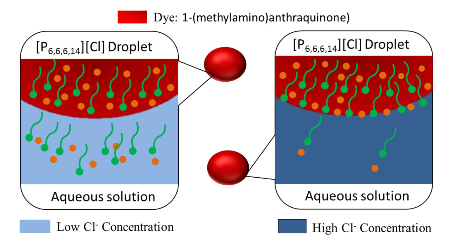
The motion of these discrete droplets was controlled by the triggered release of the  $[P_{6,6,6,14}]^+$  surfactant. In this work, the droplets were guided to specific destinations in open fluidic channels through  $Cl^-$  gradients. These  $Cl^-$  gradients were electro-generated using carbon printed or porous titanium electrodes.
