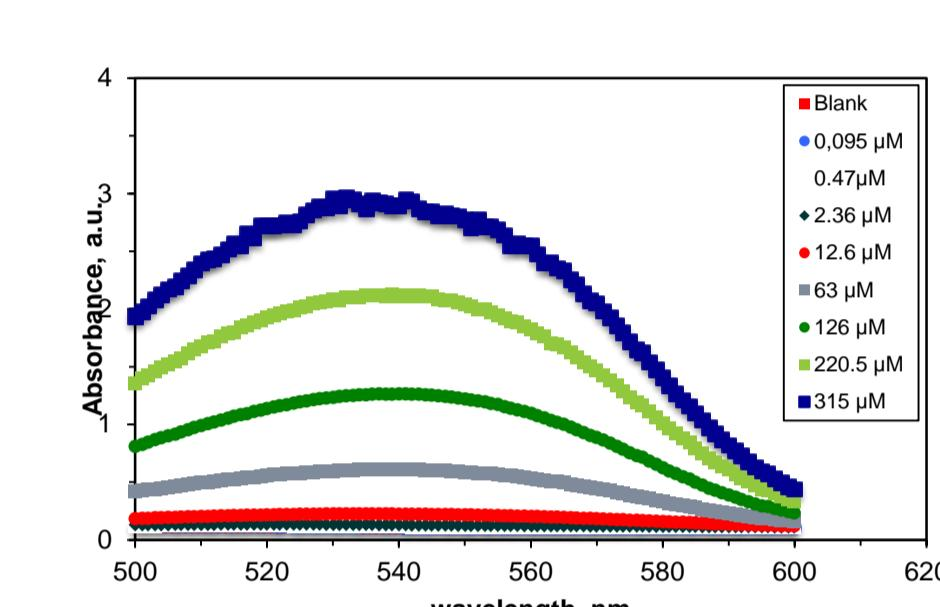
Absorbance versus wavelength for nitrite method using uv-vis spectrophotometer.
