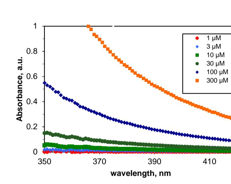
Calibration curve obtained using the yellow method from 0 to 300  $\mu\text{M}$ . Inset, lower range calibration
