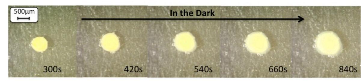
The hydrogels can reach ~49% of the fully hydrated size after 4 min of white light irradiation. After the removal of the white light the hydrogel re-swelled up to ~91% of the fully hydrated size after 11 min in the dark. This shrinking and re-swelling cycle can be repeated with great reproducibility.
