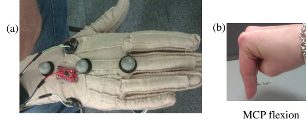
Fig. 6. (a) Placement of Vicon markers for MCP joint measurements (b) position of hand during MCP full flexion
