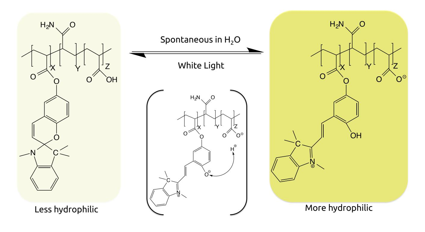
When the hydrogel is immersed in water, in the dark, the AA dissociates and the proton is taken by the SP-A to form protonated merocyanine (MC-H<sup>+</sup>)(yellow) resulting in hydrogel expansion. When exposed to white light, the MC-H <sup>+</sup> is converted back to SP-A (colourless) and some of A<sup>-</sup> gets reprotonated to AA resulting in hydrogel contraction.
